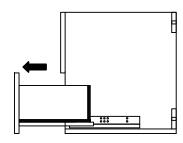
2.Pull out the bottom of the rail plastic insert and unscrew screw on side of side rail under drawer. See Page 2
